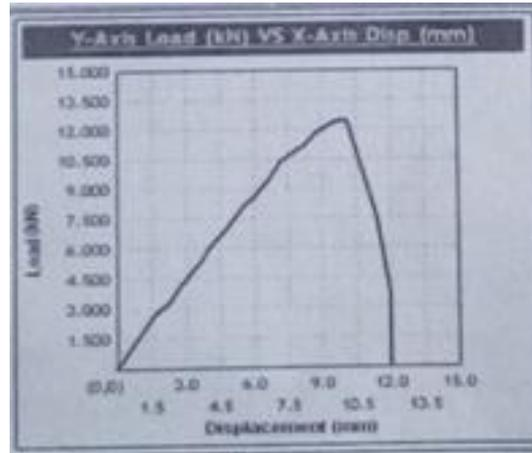
**Graph3:** 6061-6082 by using circular tip of EN31 tool
